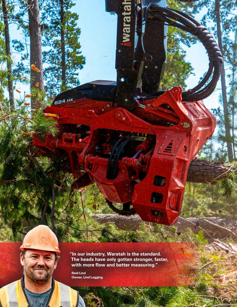
High load-bearing hanging bracket and rotator
