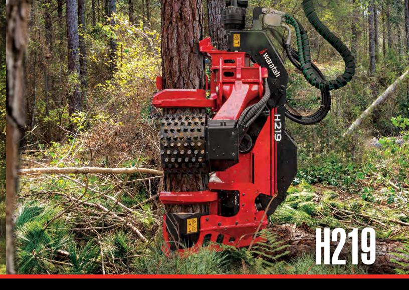
With a robust design, the H219 can handle the toughest woods. Durability is built-in with protected hoses, additional guarding and an aggressive measuring wheel. Plus, accessible servicing and a top saw option provide increased uptime and versatility.
