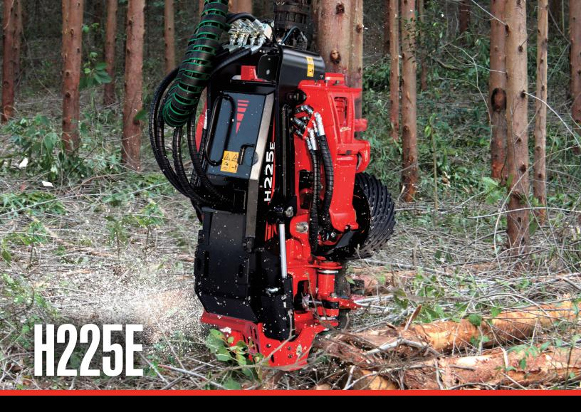
Eucalyptus is no match for the purpose-built H225E. Specifically designed for single-pass debarking, this powerful, high-capacity harvester head productively dominates in the harsh application.
