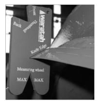
To sharpen, use a file sparingly and finish by honing the cutting edge with an oilstone.
