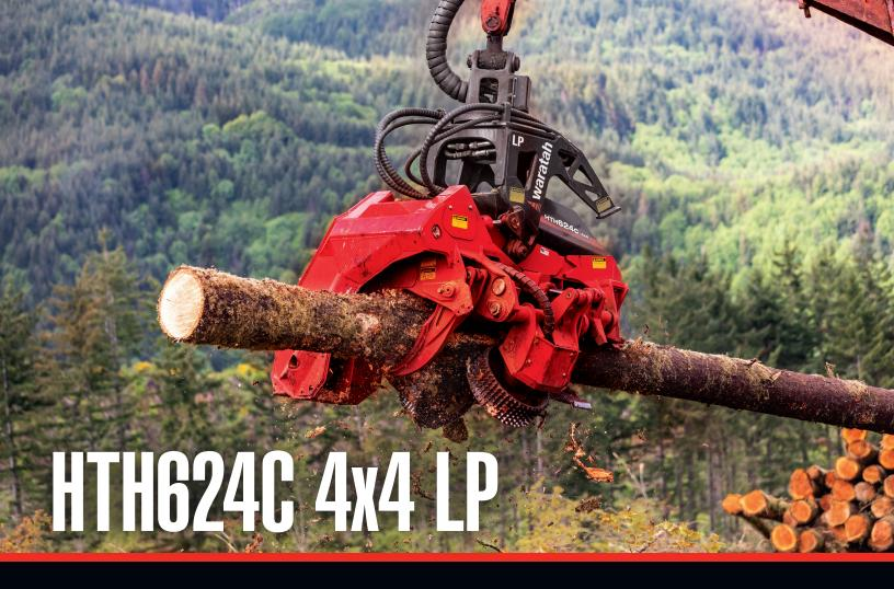
With four-wheel-drive and a wide body design, the versatile HTH624C 4x4 LP is built for exceptional delimbing, log handling and productivity. A shorter tilt frame permits loading trucks and improved reach for higher deck piles. Plus, the large delimb capacity allows operators to grab multiple logs clearing the yarder chute, shovel or manipulate larger single logs.
