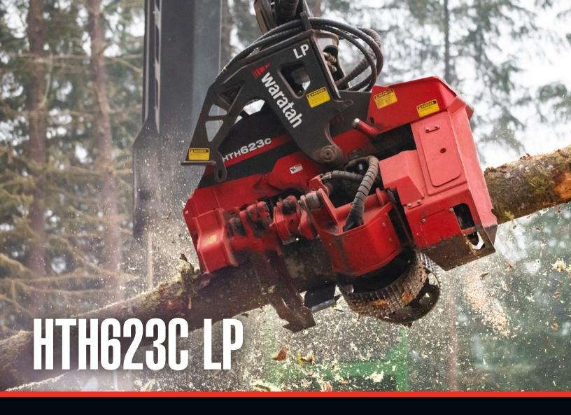
With a shorter tilt frame providing improved reach for higher deck piles, the HTH623C LP is a multi-use head built to work in tight spaces. Its large delimb opening allows for grabbing multiple logs or larger single logs, which increases efficiency and productivity for clearing the chute and loading trucks.
